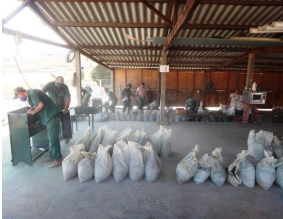
Figure 11.2.2-2 Cleaning the Riffle Splitter
