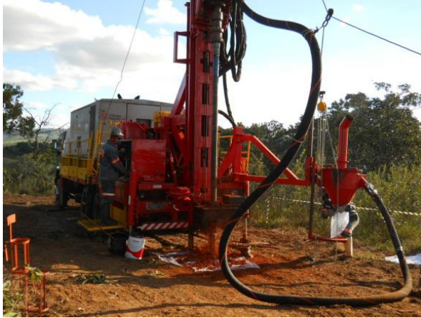
Figure 10.4-1 Fordcarro RC Drill Rig (May 2012)
