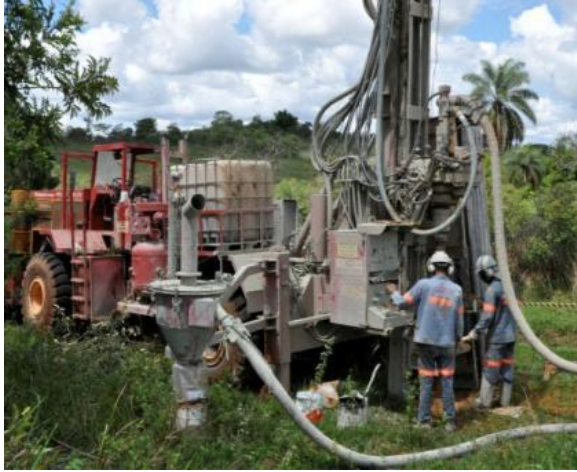
Figure 10.2-1 Foremost RC Drill Rig (Early 2011)
