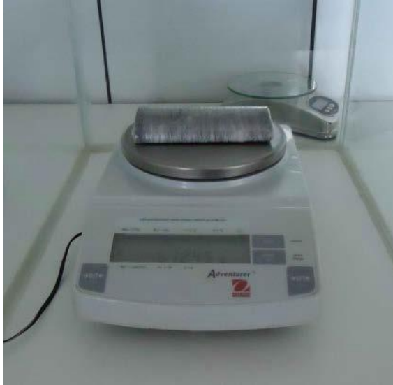
Figure 10.10-1 Wrapped Sample Weighed in Air
