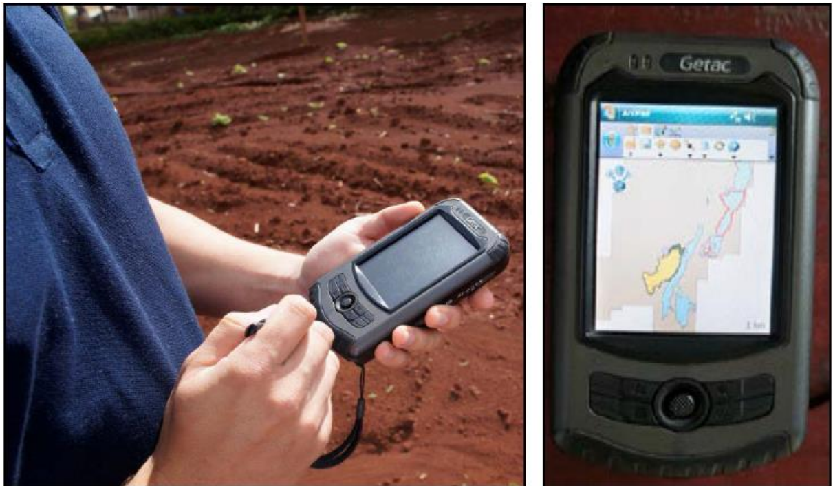
Figure 9.1.1-2 Geological Mapping using GETAC PDA's with ArcPad Software (VERDE, March 31, 2013)
