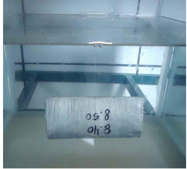
Figure 10.10-2 Wrapped Sample Weighed in Water
