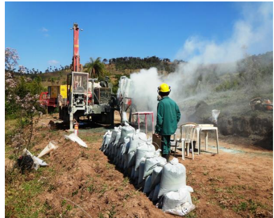
Figure 10.4-4 RC Drilling #3 - CV Target 7 (August 2012)
