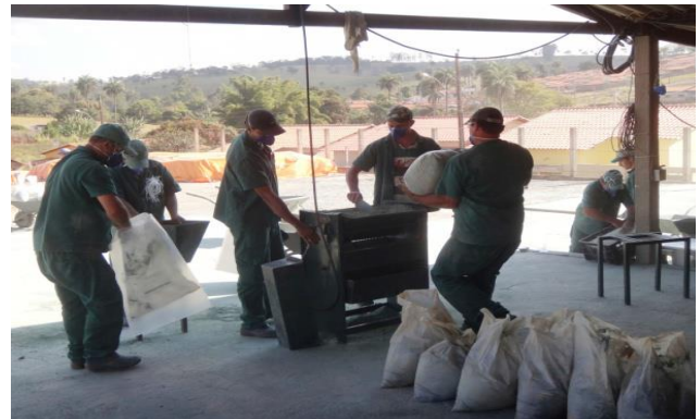
Figure 11.2.2-5 Riffle Splitting RC Samples
