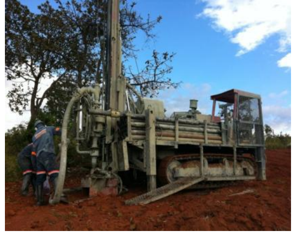
Figure 10.2-2 Explorac RC Drill Rig (Early 2011)
