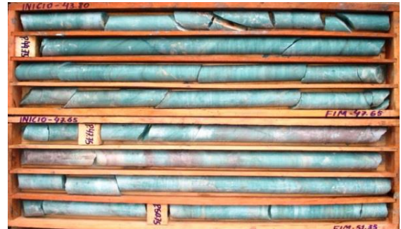
Figure 10.6-2 Diamond Core Storage
