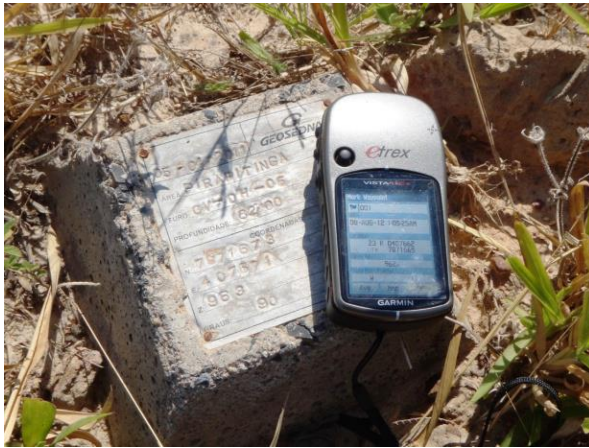
Figure 10.5-1 AMS Drill Collar Field Check
