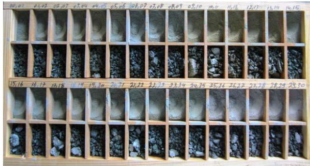
Figure 10.6-1 Reverse Circulation Sample Logging Box
